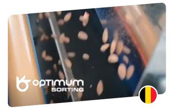
Optical food sorting machines target the removal of unwanted products from a product flow, benefitting food safety and quality by detecting foreign objects, bruised products and harmful elements. Vrije Universiteit Brussel (VUB) and Warsaw University of Technology (WUT) performed a spectroscopic study optimizing the illumination and detection parameters for nut sorting. VUB subsequently worked on an improved illumination lens design.
