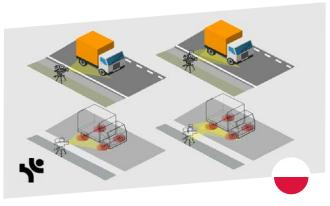
Heller Consult sp. z.o.o. enhances road safety and infrastructure maintenance through dynamic vehicle weighing (Weigh-In-Motion). In collaboration with Warsaw University of Technology (WUT) in Poland, they have developed a unique sensor system. This technology measures pavement deflection under vehicle load and recalculates axle and gross vehicle weights. The system promises more accurate and efficient road maintenance and safety management.
